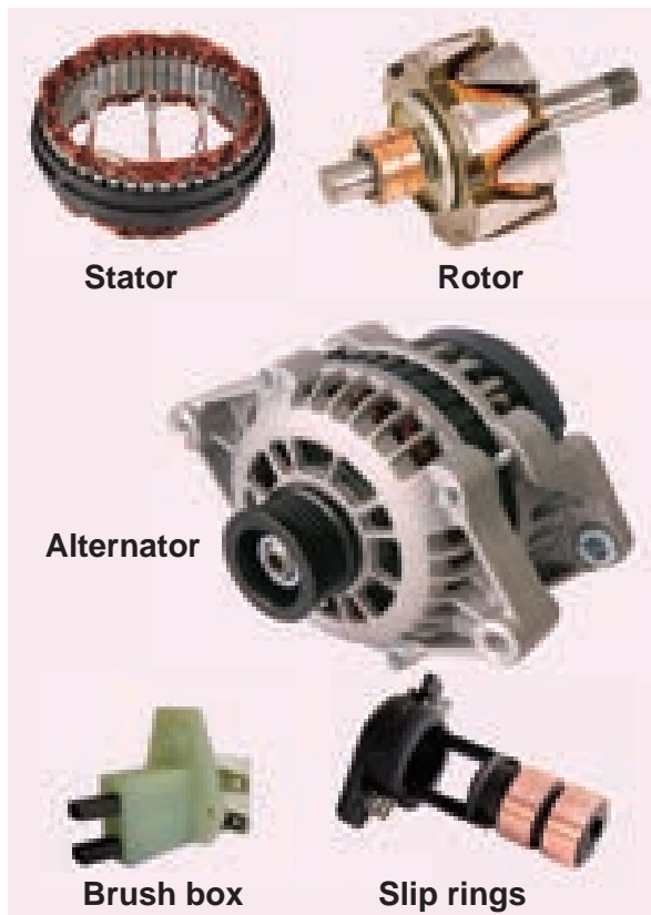
Figure 4.26 AC generator and its components
