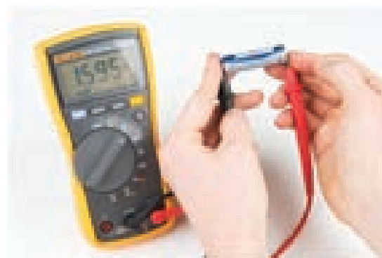
Figure 2.19 Measuring the emf of a cell
