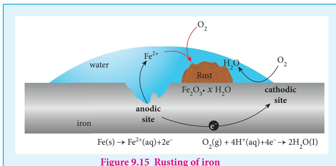
**At anode (oxidation): Iron dissolves in the anode region**
