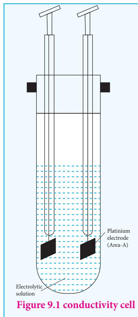
**Figure 9.1 conductivity cell**
