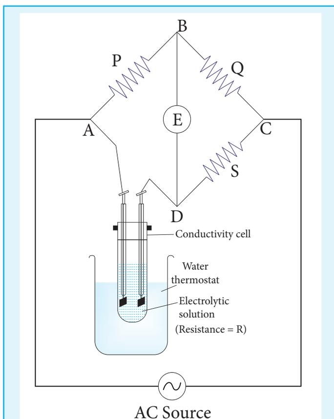
**Fig 9.3 Schematic diagram of a conductivity cell in a wheatstone bridge circuit**
