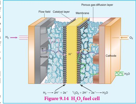
considering hydrogen – oxygen fuel cell. In this case, hydrogen act as a fuel and oxygen as an oxidant and the electrolyte is aqueous KOH maintained at 200°C and 20 – 40 atm. Porous graphite electrode containing Ni and NiO serves as the inert electrodes.
