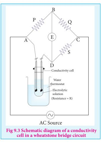
taken in it be R) as shown in the figure 9.3. An AC source (550 Hz to 5 KHz) is connected between the junctions A and C. Connect a suitable detector E (Such as the telephone ear piece detector) between the junctions 'B' and 'D'.
