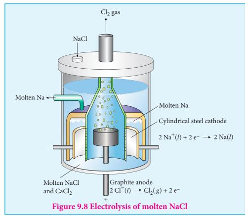
attached to the positive end is called the anode. Once the key is closed, the external DC power supply drives the electrons to the cathode and at the same time pull the electrons from the anode.
