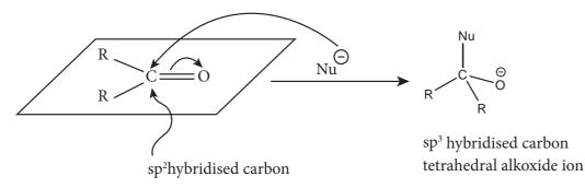
The tetrahedral intermediate can be protonated by water or an acid to form an alcohol.
