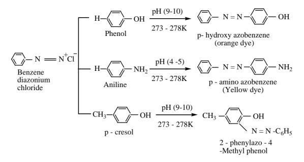
Aryl fluorides and iodides cannot be prepared by direct halogenation and the cyano group cannot be introduced by nucleophilic substitution of chlorine in chlorbenzene. For introducing such a halide group, cyano group -OH, NO<sub>2</sub> etc.. benzenediazonium chloride is a very good intermediate Diazo compounds obtained from the coupling reactions of diazonium salts are coloured and are used as dyes.
