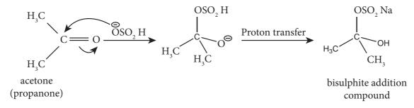
This reaction finds application in the separation and purification of carbonyl compound. The bisulphate addition compound is water soluble and the solution is treated with mineral acid to regenerate the carbonyl compounds .
