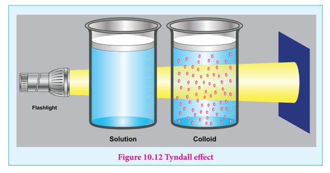
But when light passes through colloidal solution, it is scattered in all directions. This effect was first observed by Faraday, but investigations are made by Tyndall in detail, hence called as Tyndall effect.
