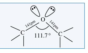
' bonds. The C-O-C bond angle is slightly greater than the tetrahedral bond angle due to the repulsive interaction between the two bulkier alkyl groups.
