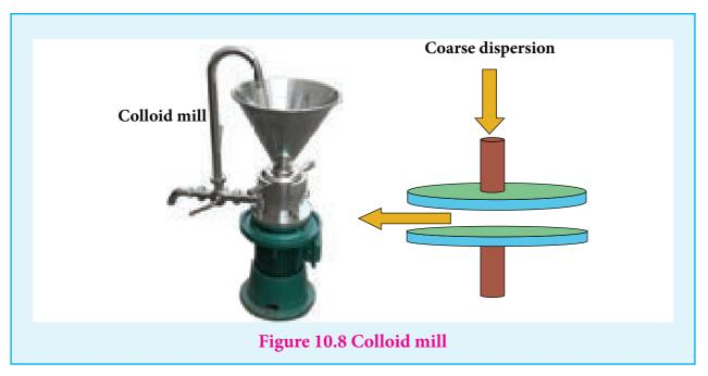
The colloidal particles of required colloidal size is obtained by adjusting the distance between two plates.
