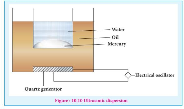
Claus obtained mercury sol by subjecting mercury to sufficiently high frequency ultrasonic vibrations.
