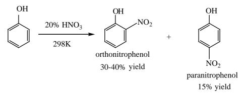
The ortho and para isomers are separated by steam distillation, as o-nitro phenol is slightly soluble in water and more volatile due to intra molecular hydrogen bonding, whereas p-nitro phenol is more soluble in water and less volatile due to intermolecular hydrogen bonding.
