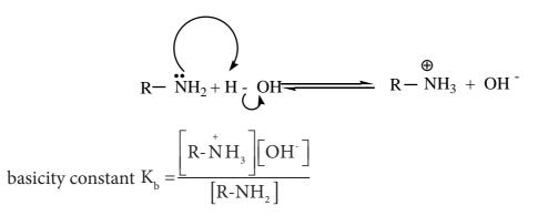
The basicity constant Kb gives a measure of the extent to which the amine accepts the hydrogen ion  $(H^+)$  from water,
