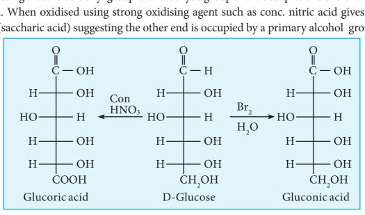
5. Glucose is oxidised to gluconic acid with ammonical silver nitrate (Tollen's reagent) and alkaline copper sulphate (Fehling's solution). Tollen's reagent is reduced to metallic silver and Fehling's solution to cuprous oxide which appears as red precipitate. These reactions further confirm the presence of an aldehyde group
