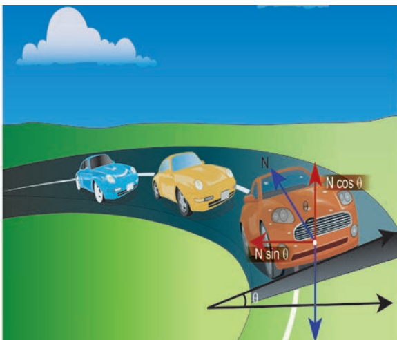
Figure 3.44 Outer edge of the road is slightly raised to avoid skidding
